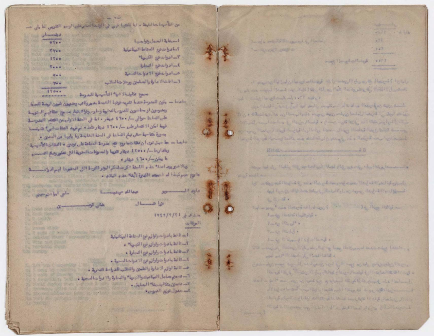
IIIs. 500/-1. One 6" contre 5' bed lathe (motor-driven) 200/-2. One smaller belt driven lathe 300/-3. One shaping machine-12" 4. Emery grinding machine (12" whoels) 50/-Tellustrates the planting the state of 5. Helt driven grinding machine 90/-6. Drilling machine (Notor Driven)
