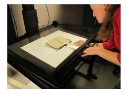
Image 22 Gently lower glass while positioning the page with the matboard tool
